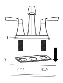
Place the faucet body (#1) and gasket (#2) on top of the sink and insert through the installation holes.
