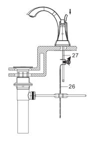
9.Insert the lift rod (#27) through the pop-up hole on the faucet. Underneath the sink insert the lift rod (#27) through the lift rod strap (#26). Tighten the thumb screw on the lift strap.Note: be sure to ensure there is enough room to lift the lift rod up and down to open and close the drain.
