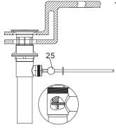
7.Ensure the ball rod (#25) is inserted through the drain stopper base hole. See diagram for visual.
