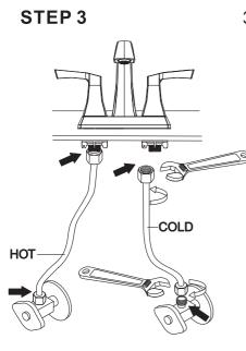
3. Connect the water supply lines to the tail pipes of the faucet and to the hot and cold water supply valves. Secure and tighten with an adjustable wrench. Caution: Be careful not to mix up the hot and cold supply lines. Check all connections (shown with arrows in the image) for leaks. Re-tighten if necessary. Do not over tighten!
