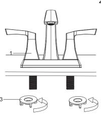
2. From under the sink, secure the faucet with Mounting Nuts (#3). Tighten the lock nut by hand. Do not over tighten!
