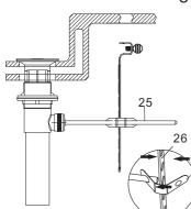
8. Place one end of the spring clip (#28) on the end of the ball rod (#25). Insert the ball rod through the hole on the lift rod strap (#26), then slide the other end of the spring clip (#28) over the ball rod (#25). See diagram for visual.
