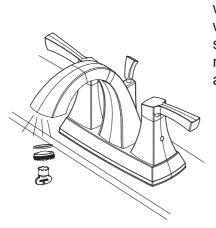
4. Remove the aerator using the aerator wrench. Turn the faucet handle all the way on, turn on hot and cold water supply and flush water lines for one minute. Reinstall aerator using the aerator wrench.
