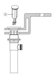
6.Insert drain stopper 4 into the drain.
