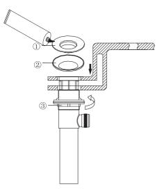
5.Place a bead of silicone or plumbers putty as shown on the drain opening of the sink. Thread the top (1 2) into the drain. Secure the drain by tightening the nut (3) underneath the sink.
